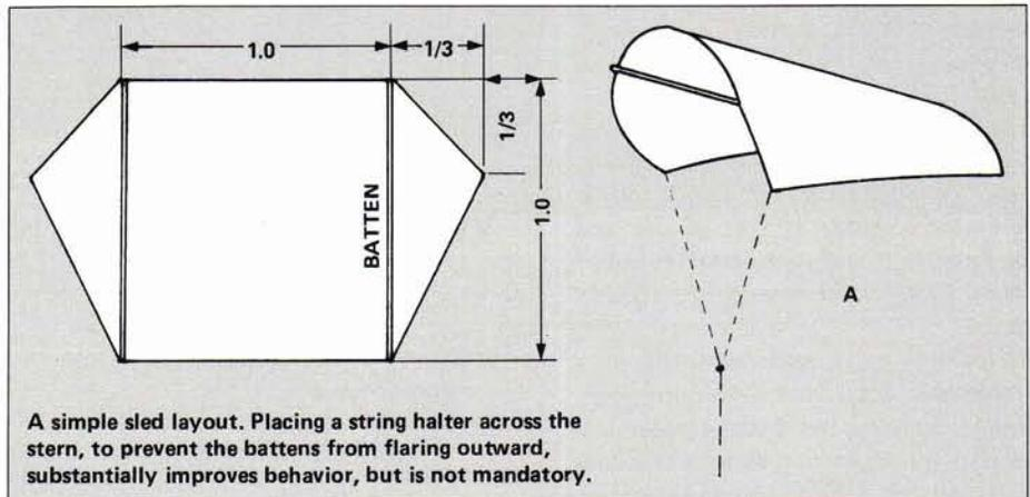
long as you maintain sufficient tension. So it is with the leading edge of a sled. A properly constructed sled is as reliable as any other kite, and more so than many. It does not require a tail or drogue.
